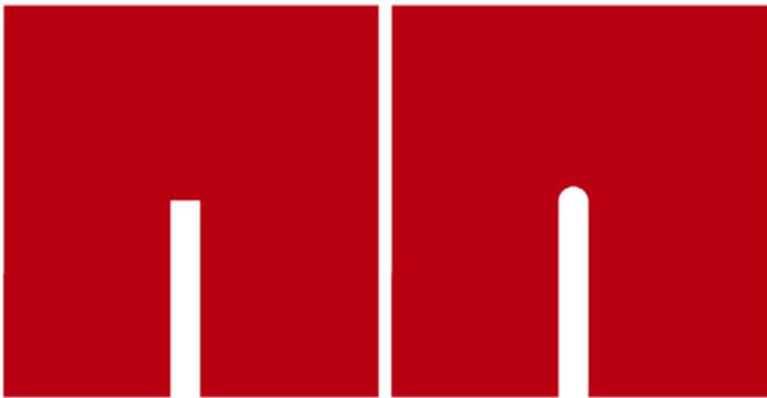
Figure 6-17. Submodel geometries for the slit bottom (plane and curved bottom). The width of the slit is 160 µm, and the entire submodel geometry is approximately 2 × 2 mm 2 (Unosson 2017).
