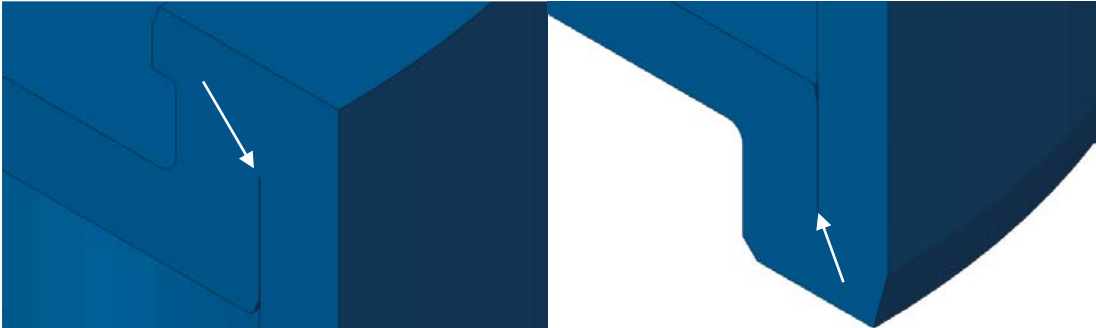
Figure 6-16. The FE model of the slits at the top of the canister (left) and welded base (right) without the root defect. The tips of the arrows indicate the bottoms of the slits where the worst strains and stresses usually occur.
