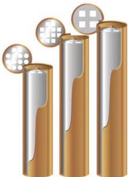
Figure 1-2. An artist rendition of the copper/iron canisters: (left) VVER 440 type, (middle) BWR type, and (right) EPR type (Raiko 2013).
